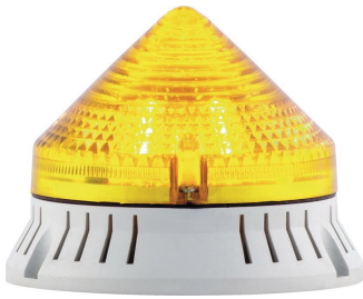
SIRENA CTL A 900 LED-SMD blink/dauer + akustik, gelb, 12/24V, ACDC, IP30
