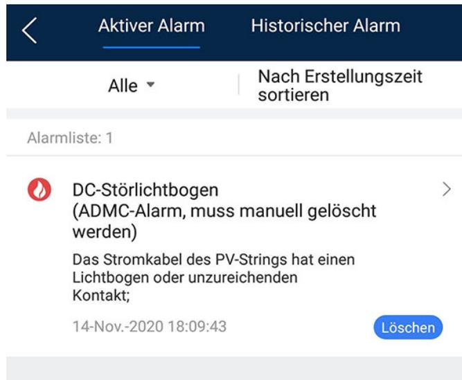
● **Methode 2:** FusionSolar Smart PV-Managementsystem
