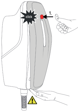
Fig. 18: Colocar o painel frontal - 1
