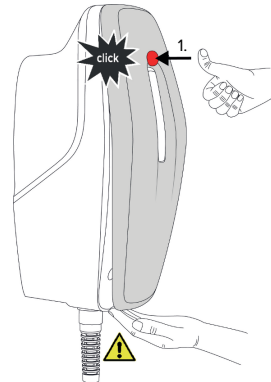
Fig. 18: Anbringe front cover - 1
