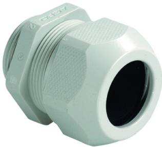
AGRO Kabelversch. SYNTEC PA6 Pg48 hellgrau RAL7035 Ø 32,0 - 44,0mm (UL 44)
