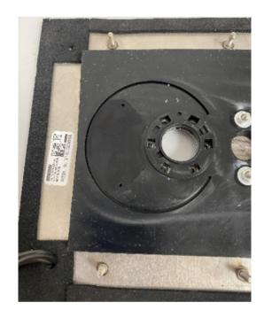
11. Replace the amplifier and replace the clamps, screw them on with the hexagon sockets and reconnect the flexible hoses or connectors as they were at the beginning.
