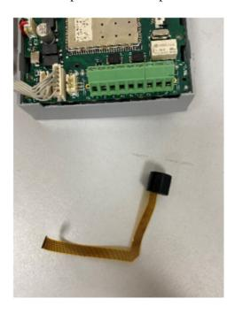
6. Insert the new microphone from the front. Make sure that the part fits correctly with the corresponding tab.
