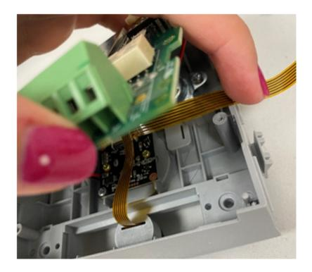
8. Once the ribbon cable has been inserted and correctly aligned, close the black tabs with the screwdriver. Pull the ribbon cable slightly to ensure that it is securely fastened..
