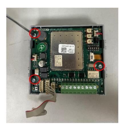
4. We have to disconnect the flat cable from the microphone. To do this, use a thin flat-blade screwdriver to press the black retaining tabs on each side of the microphone. Once opened, the ribbon cable can be released. The microphone can then be removed from the front.
