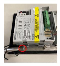
Remove the cable clamps and disconnect any connectors or flex connectors that are connected to the amplifier.
