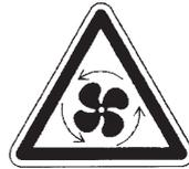
After switching off the fan, the impeller continues to run for some time. To avoid risk of injury, refrain from reaching into the fan until it has come to a standstill.
